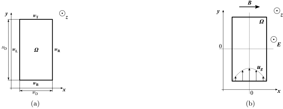
Figure 1: Diagram of the model spatial configuration: (a) boundaries and dimensions; (b) magnetic field vector \mathbf{B} , electric field vector \mathbf{E} , profile of the gas velocity \mathbf{u}_g .
